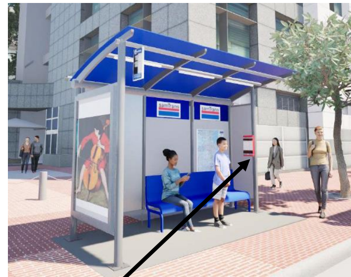
Placement within bus shelter: within the structure so passengers under the shelter can read the sign
