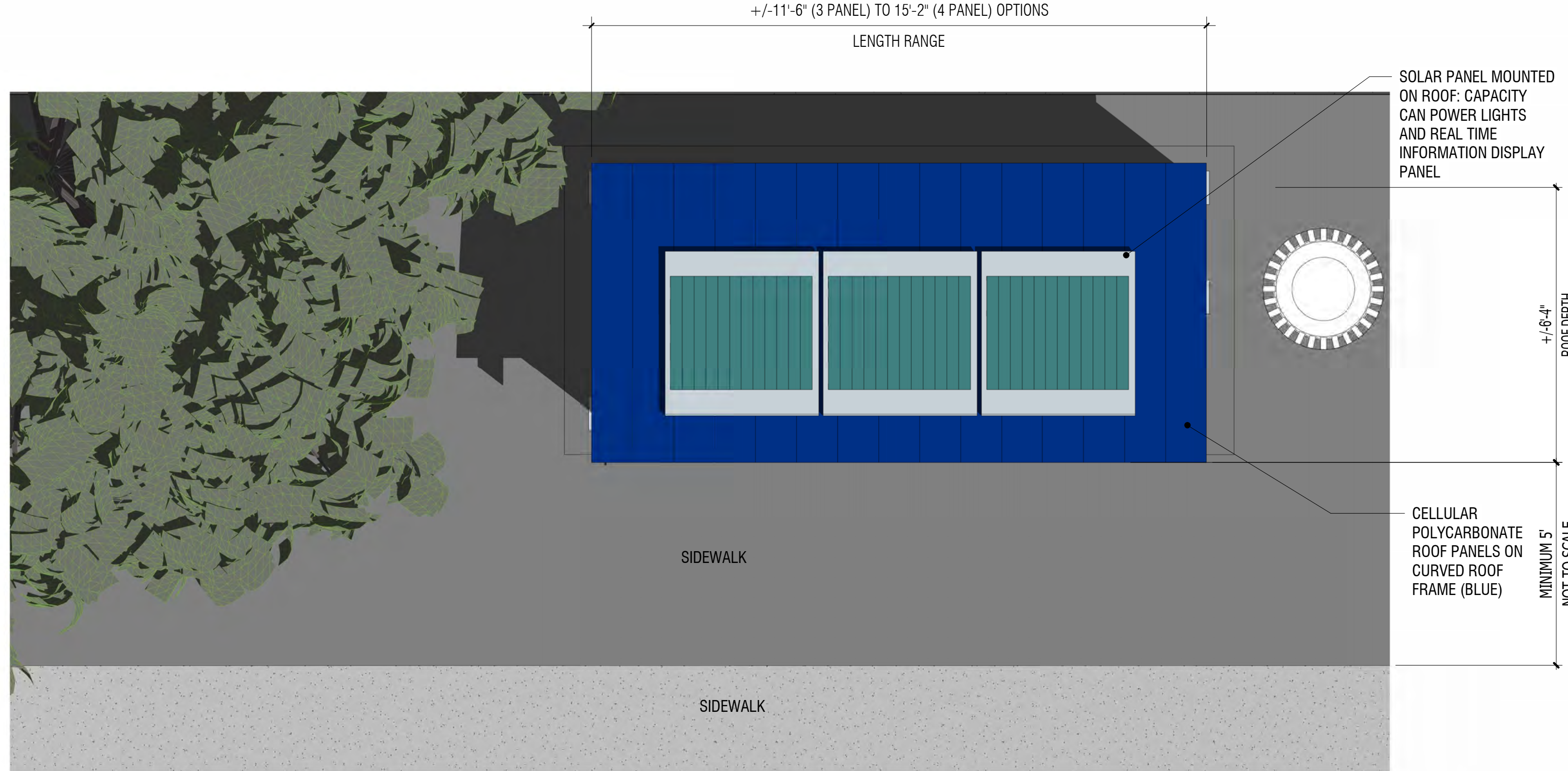
ROOF PLAN 1 SCALE: 1/2" = 1'-0" 1 A01
