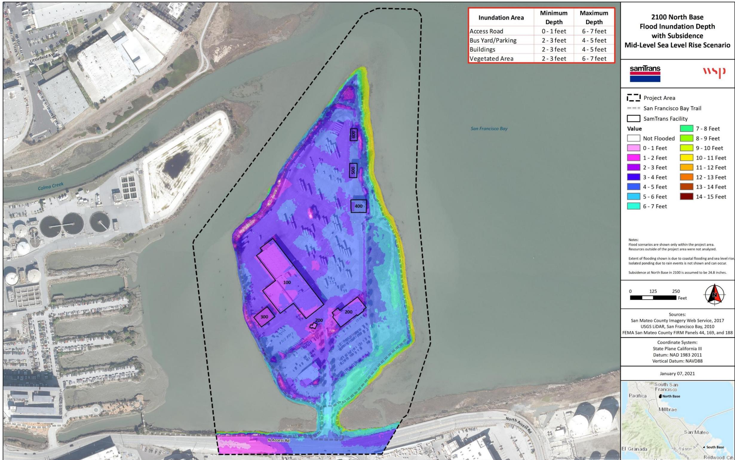
Figure 9. 2100 North Base Flood Inundation Depth with Subsidence High-End SLR Scenario
