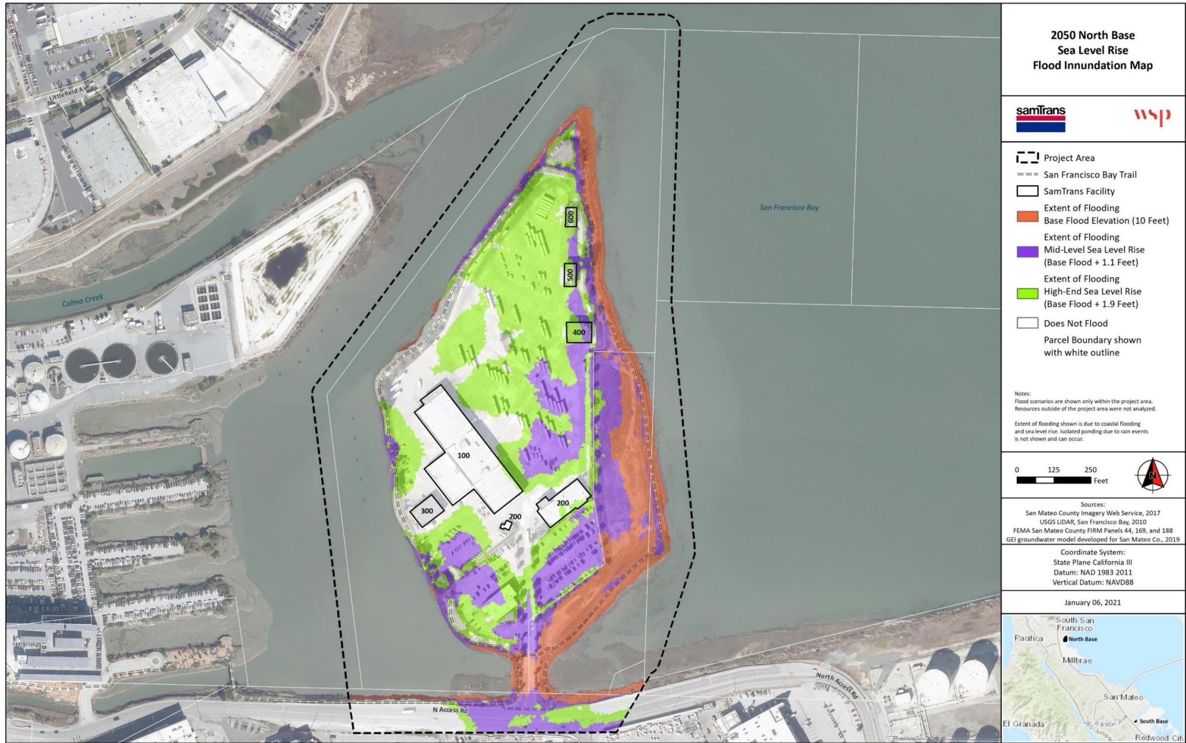
Figure 5. 2050 North Base Flood Inundation Depth with Subsidence Mid-Level SLR Scenario
