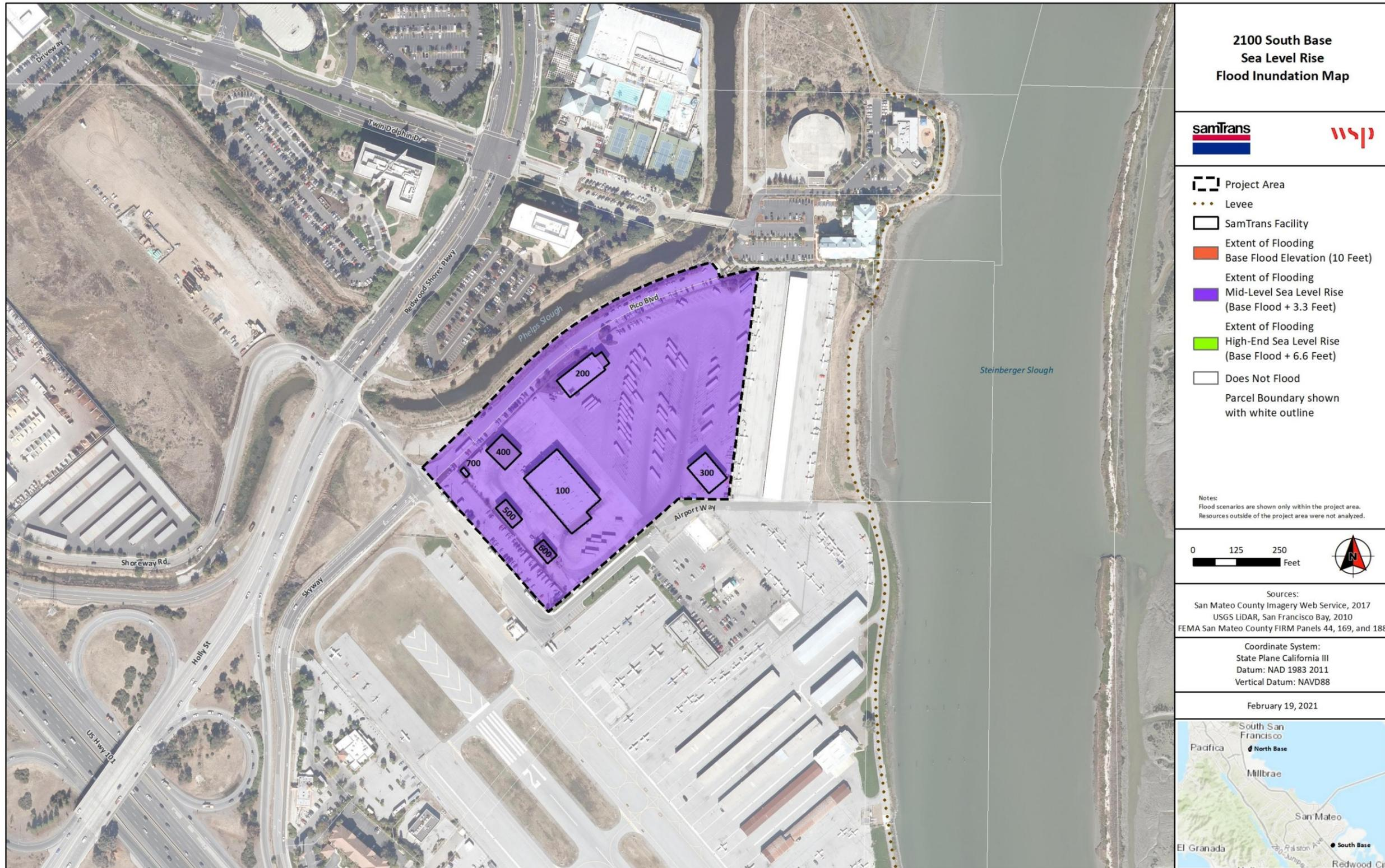
Figure 14. 2100 South Base Flood Inundation Depth with Subsidence Mid-Level SLR Scenario
