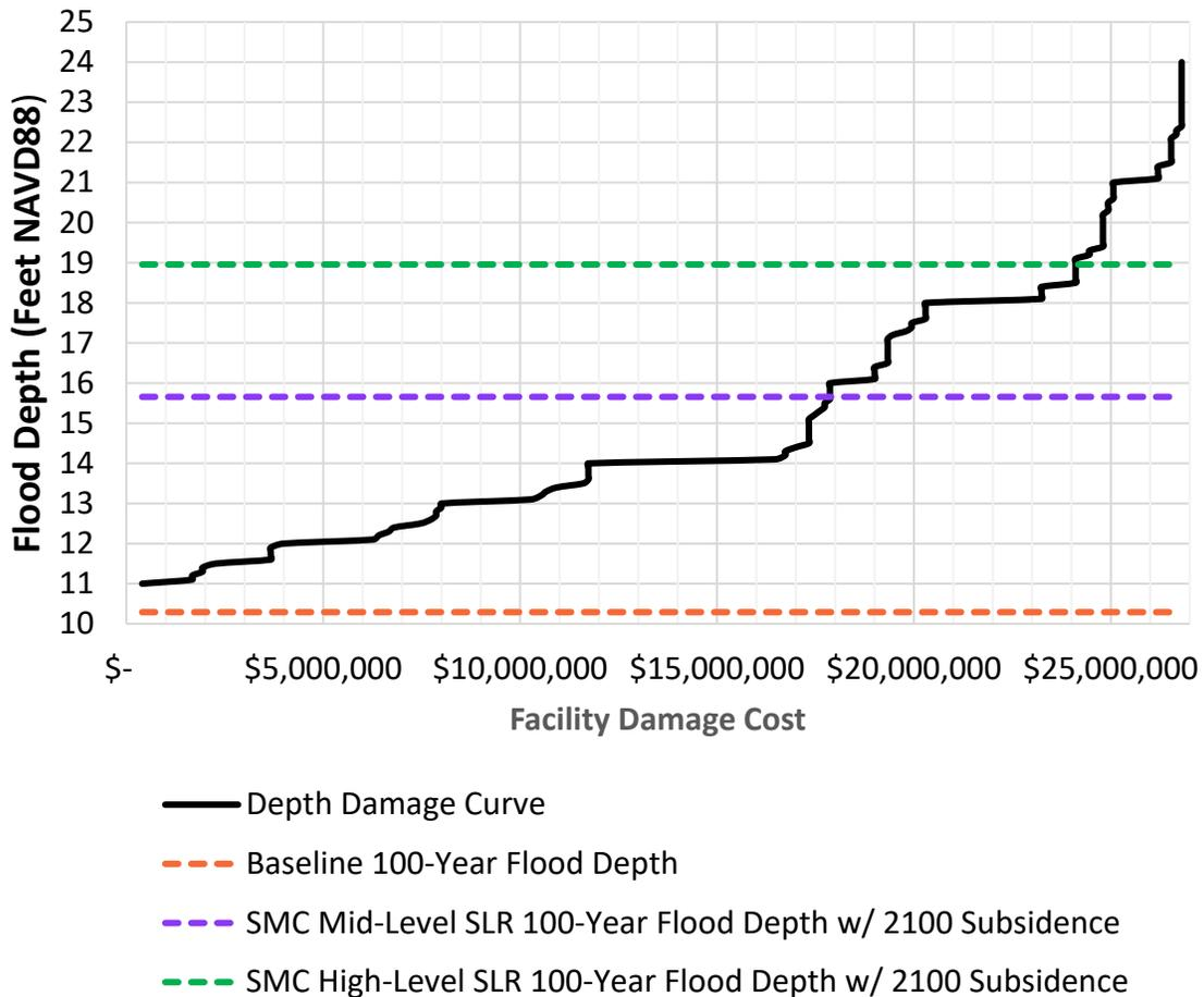
**Figure 27. Facility Damage Costs by Flood Depth**
