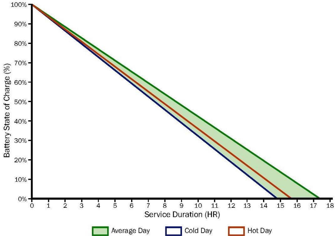
**Figure 22: BEB Change in SOC Under Different Temperature Conditions**
