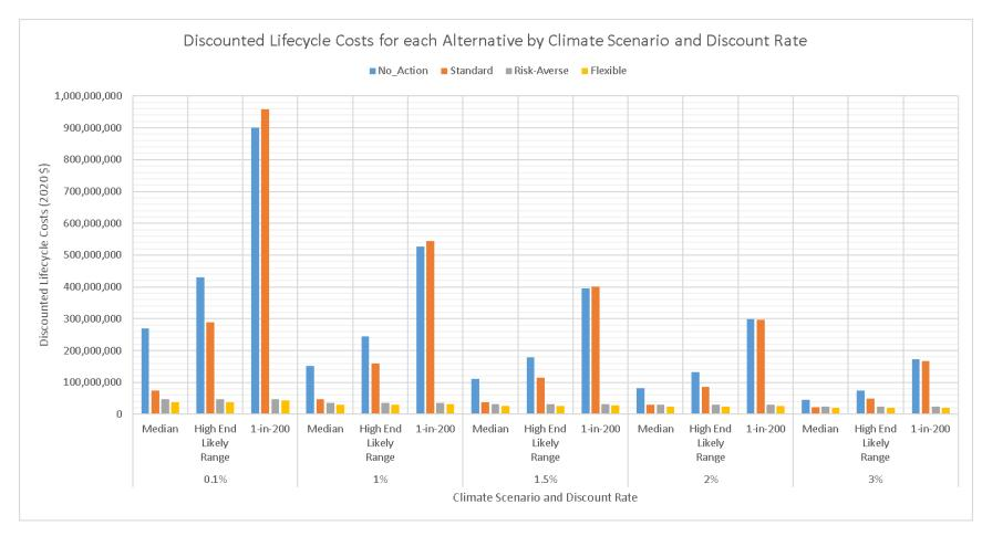
Figure 30. Discounted Lifecycle Costs for each Alternative by Climate Scenario and Discount Rate (50<sup>th</sup> Percentile)
