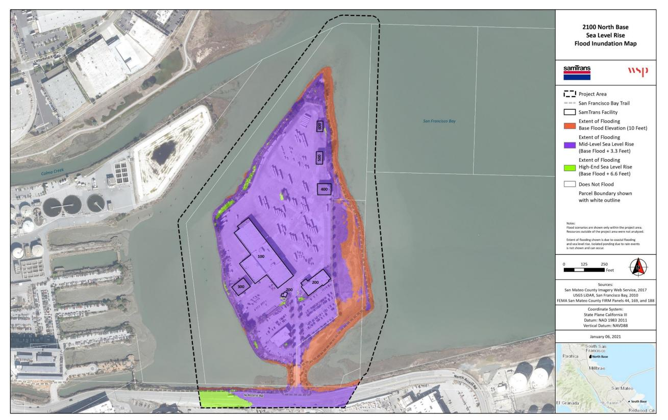
Figure 8. 2100 North Base Flood Inundation Depth with Subsidence Mid-Level SLR Scenario
